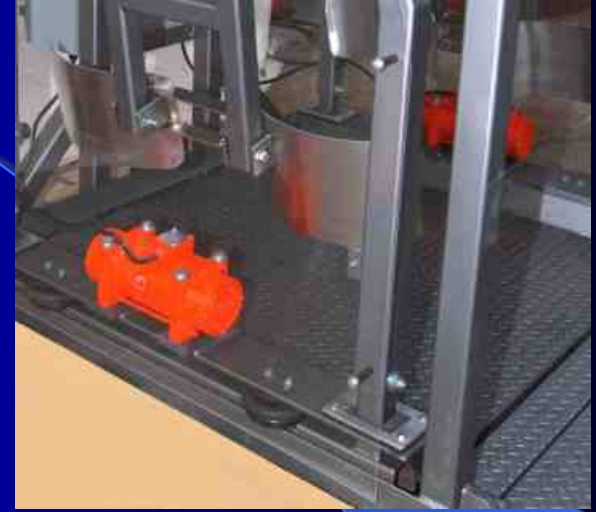
Self contained vibration system
