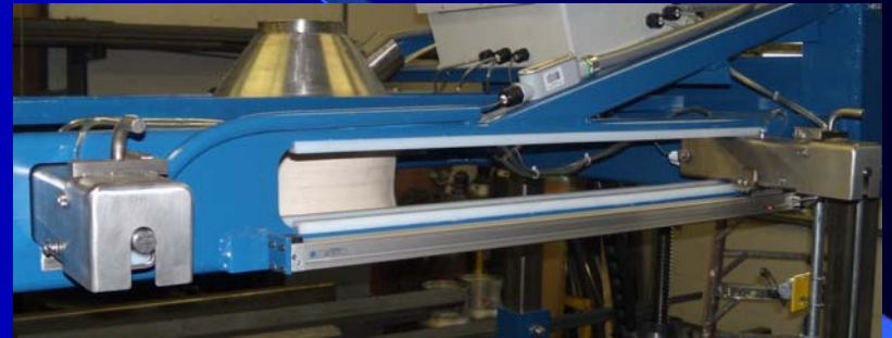
BAG HOOKS SHOWN IN THE BAG FILL POSITION
