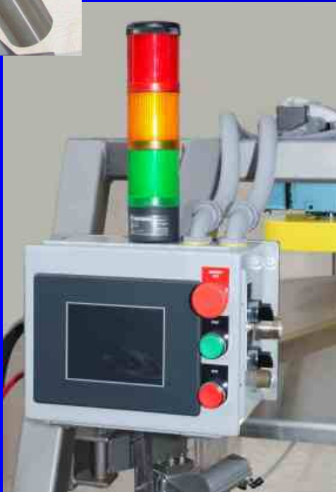
Stack lights to alert operator
