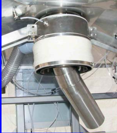
Removable chute for filling totes, drums, or bulk bags all on the same machine.
